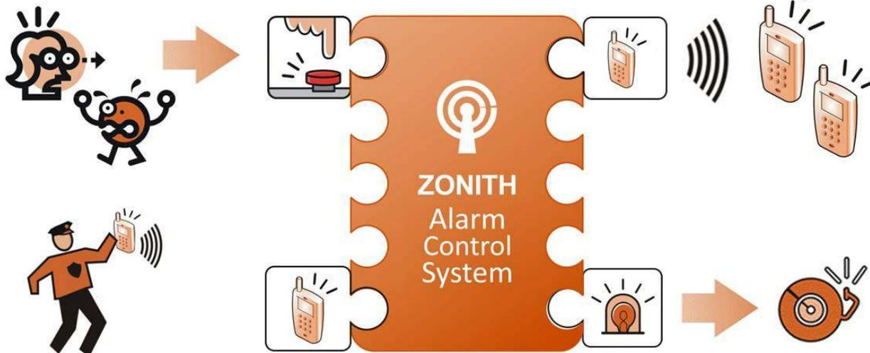
*Emergency alarms raised by security guard MOTOTRBO radios are sent to the ZONITH Alarm Control System.*
