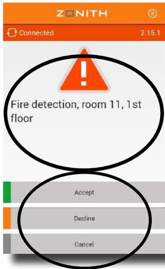
The Android App can receive alarms from all sources which have been handled by the ZONITH ACS. The user can decide to accept, decline, or cancel the alarm at the push of a button on the screen.
