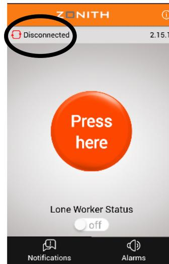
The Android App can be installed on any SmartPhone with Android 4.0 or higher. The App runs over the WiFi network and the connection status is displayed on the screen. If the connection is lost the App warns the user.
