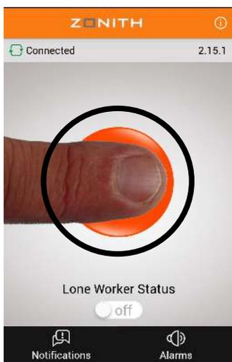
Emergency alarms can be raised by pushing the red-button on the touch screen. Once the Alarm has been sent successfully, a message is displayed on the screen.
