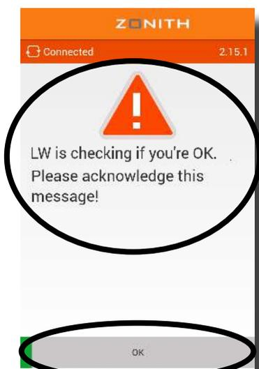
The Lone-Worker protection service can be activated manually or automatically based on the time of day or the inside/outside location of the SmartPhone. The Lone-Worker protection service works in conjunction with the ZONITH RTLS safe/un-safe area concept.
