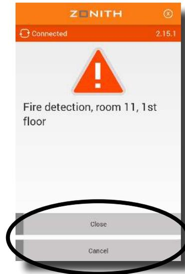
Declining an alarm notifies the ACS, which redirects the alarm message to the next person or group of persons, for acceptance. After the incident has been handled the user can close the alarm. The response will be logged in the ZONITH ACS.
