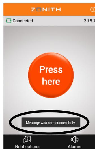
Via the ZONITH Alarm Control System (ACS) software package, Emergency alarms from SmartPhones can be dispatched to a variety of other medias including TETRA and MOTOTRBO radios, WiFi/DECT phones, GSM mobiles, monitors and other Android SmartPhones.
