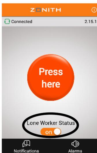
The Lone-Worker protection service monitors personnel by sending "alive-check" messages to their phone. If a person can't reply for any reason the Lone-Worker protection service will immediately notify rescue staff to ensure action is taken.
